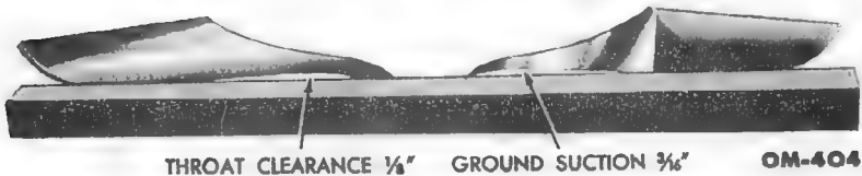
Fig. 78—Plow Shares—Ground Suction and Throat Clearance
